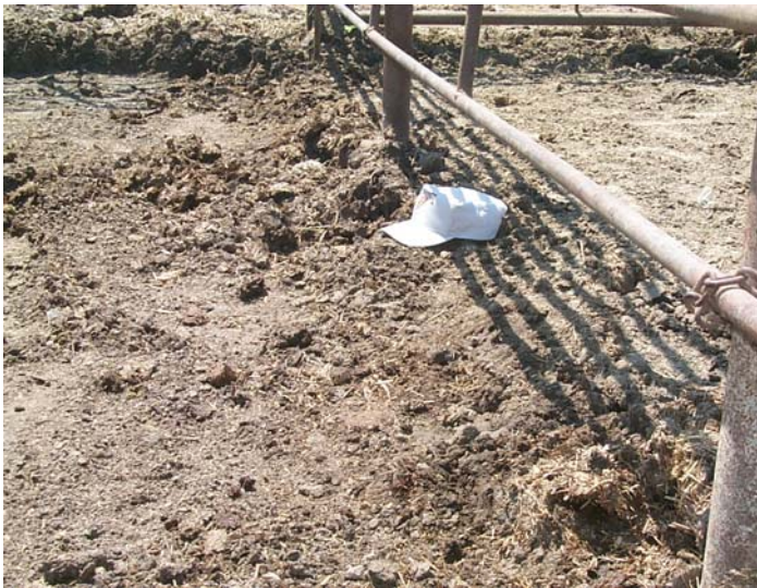
Photo 3. Erosion of surface of control pen vs. fly ash pen after three years in place.
