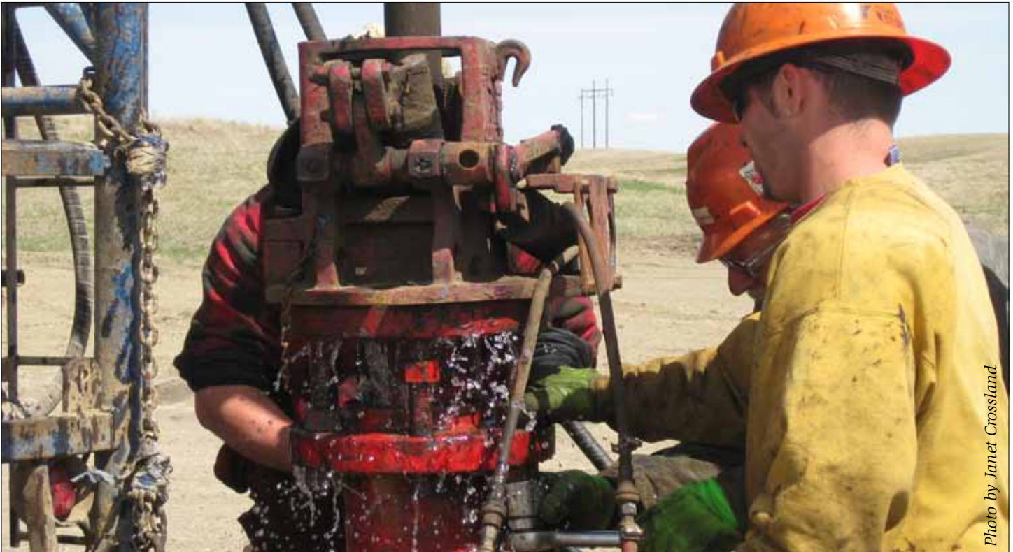
The crew of Eagle Well Service drill into a deep lignite seam in preparation for CO 2 injection and storage.
